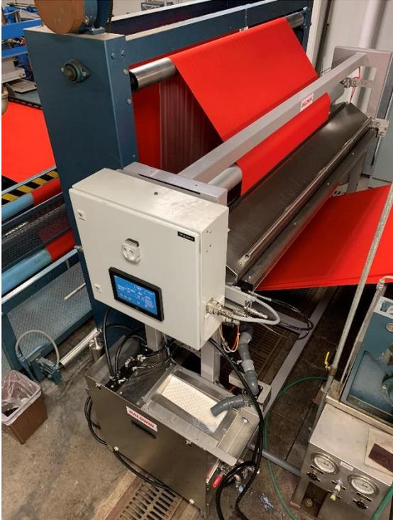
Baldwin's non-contact spray technology Texcoat G4. (Photo: Baldwin)
